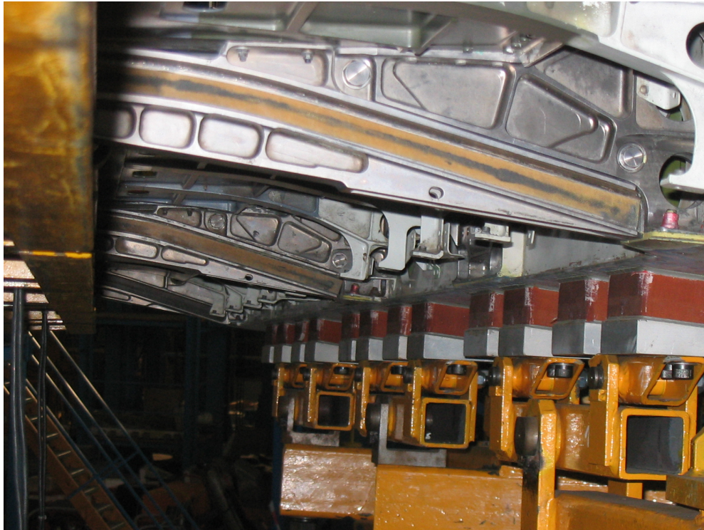
Figure 1 - MAFT: dummy flaps (beams) to load fixed flap tracks
