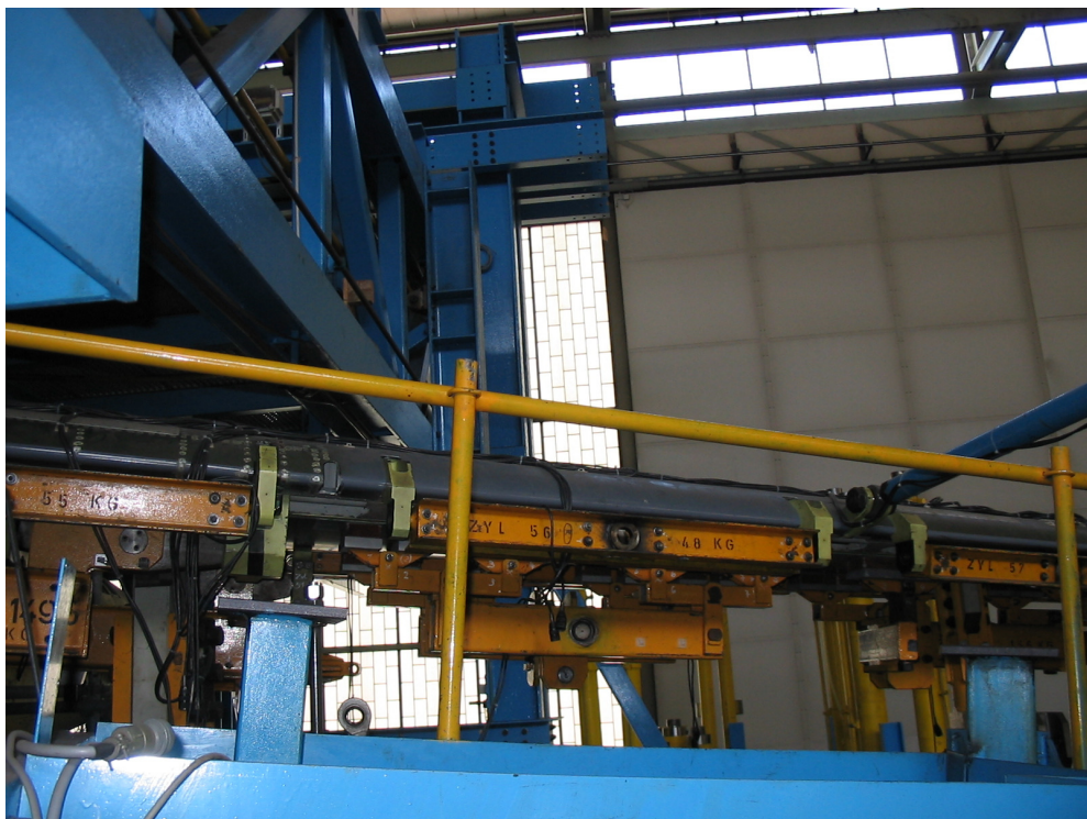
Figure 2 - MAFT: dummy slats (beams) to load wing box
